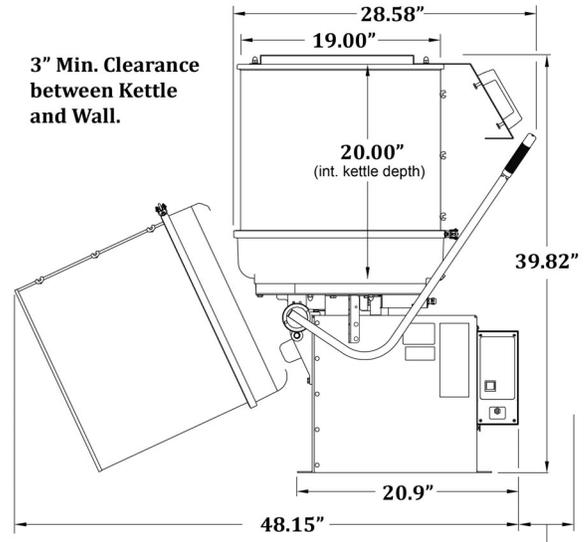
3" Min. Clearance between Kettle and Wall.
